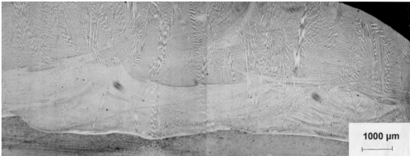
Fig. 10 Optical micrograph of a cross section of an Inconel alloy clad onto a steel substrate. Source: Ref 32
